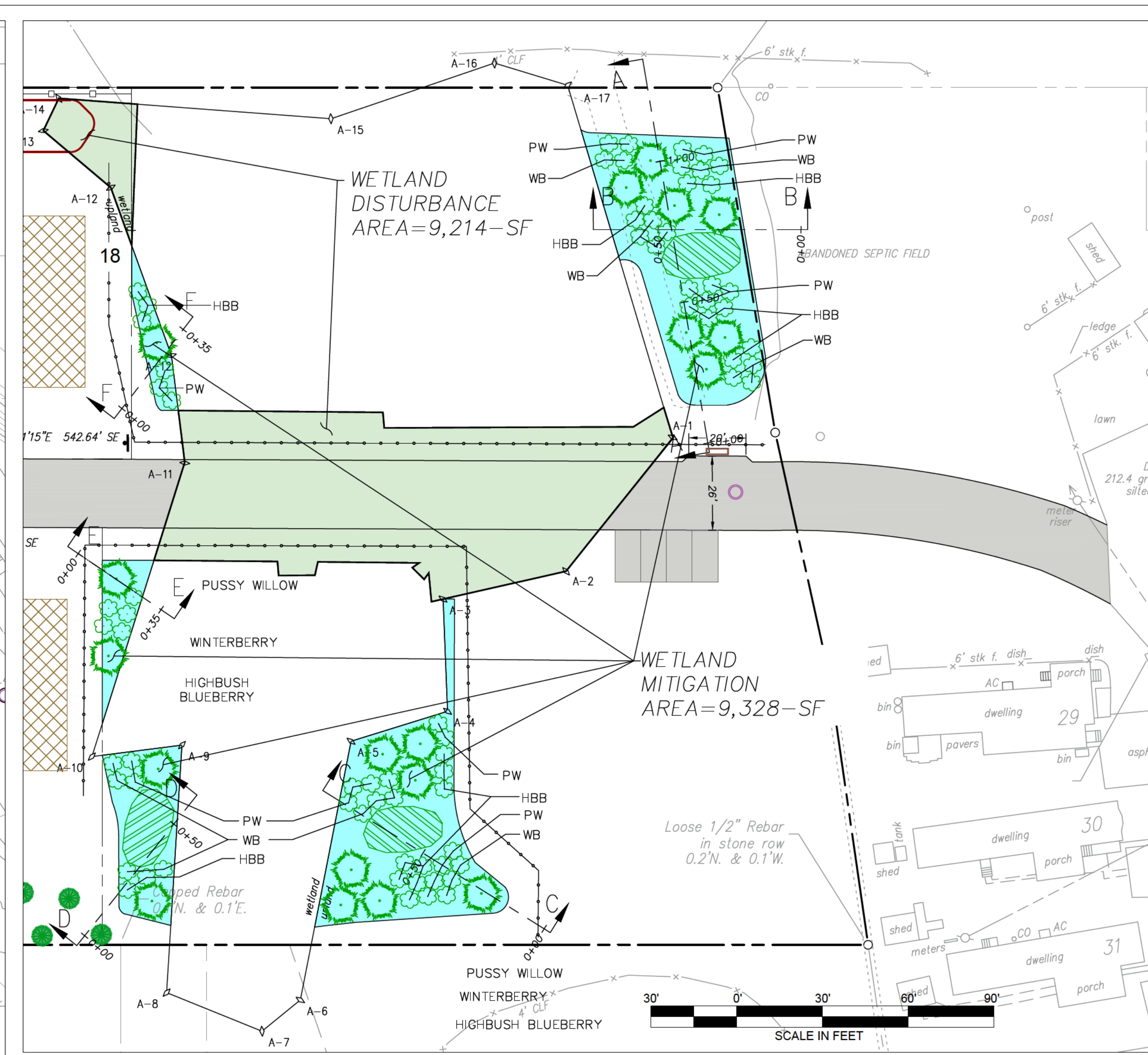
WETLAND MITIGATION AREA - PLANTING PLAN SCALE: 1" = 30"
