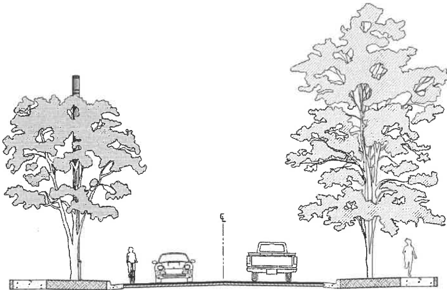
Figure 8: Freestanding Small Cell Pole in Amenity Zone of ROW
